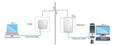
1. Press the Pair button on P200 for 2-3 seconds and then release it. The Power LED on P200 starts blinking, which indicates the P200 is ready for pair auto-negotiation.
