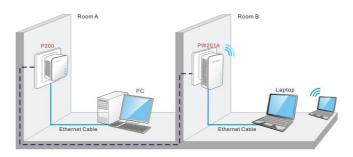
Figure 1-3 Establish a Powerline Network
