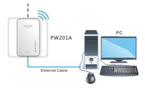
Figure 1-6 Terminal Connection
