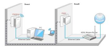
Figure 1-4 Connect Powerline Network to Internet
